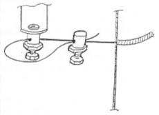
The inner cable then continues through the 1/16" nose cone hole, passes through a floating ferrule and then through a second ferrule attached to the end of the lock lever. It is secured to the lever ferrule by a grub screw. The inner cable then loops back on itself and passes back through the first floating ferrule where it is again secured with a grub screw. It is important that the inner cable is not under any tension.
