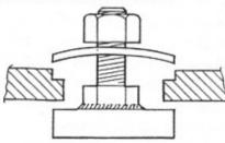
Weld a 1 5/8" long piece of 3/8" Dia. steel rod to the head of a 3/8"Dia. bolt.
