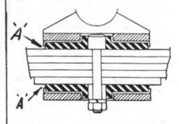
There should be clearance between the steel locating plates and the top and bottom spring leaves at location 'A'.
